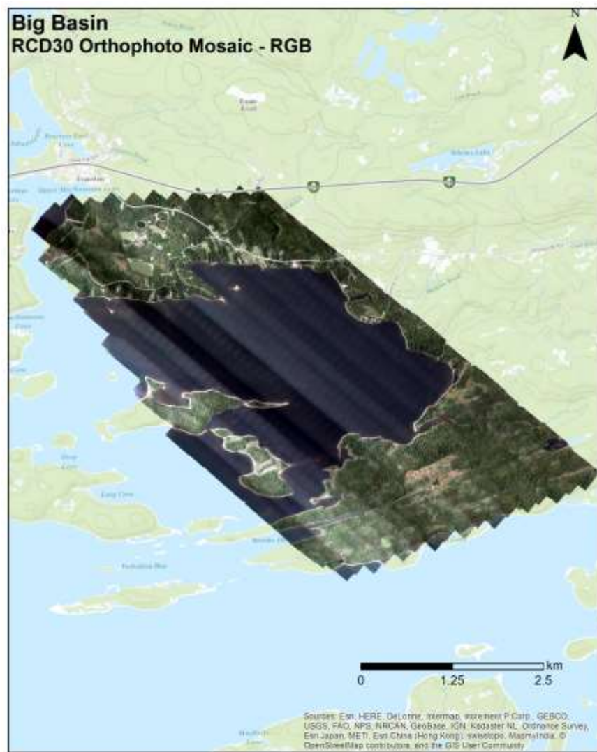
Figure 2.14: Example of the RCD30 orthophoto mosaic in true colour RGB.
