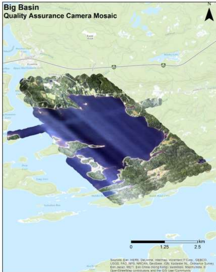
Figure 2.13: Example of the 20cm QA orthophoto mosaic used in the bottom classification.
