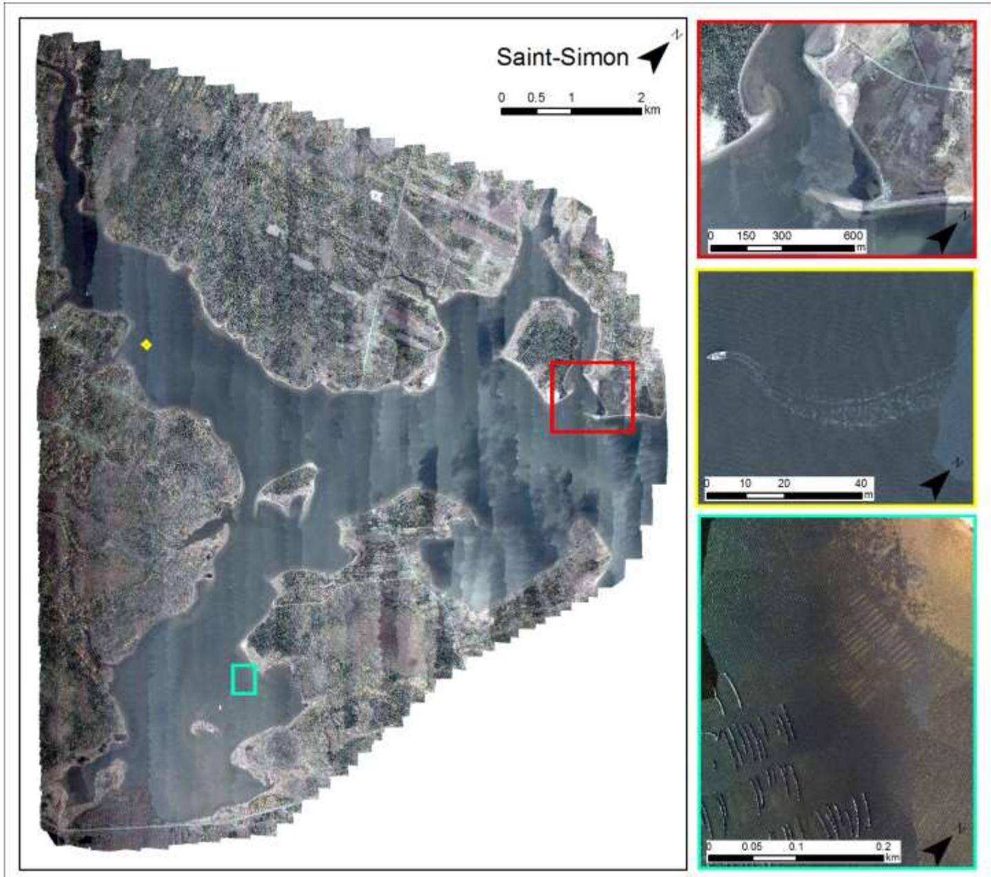
Figure 3.15: Saint-Simon Bay Orthophoto Mosaic from Oct. 24, 2015 showing the whole study area, and insets beside which are matched to the larger figure by border colour. The insets, from top to bottom, highlight submerged vegetation, the AGRG boat conducting ground truth surveys during the survey, and aquaculture, both submerged and floating, in the southern part of the bay (same extent as Figure 3.12).
