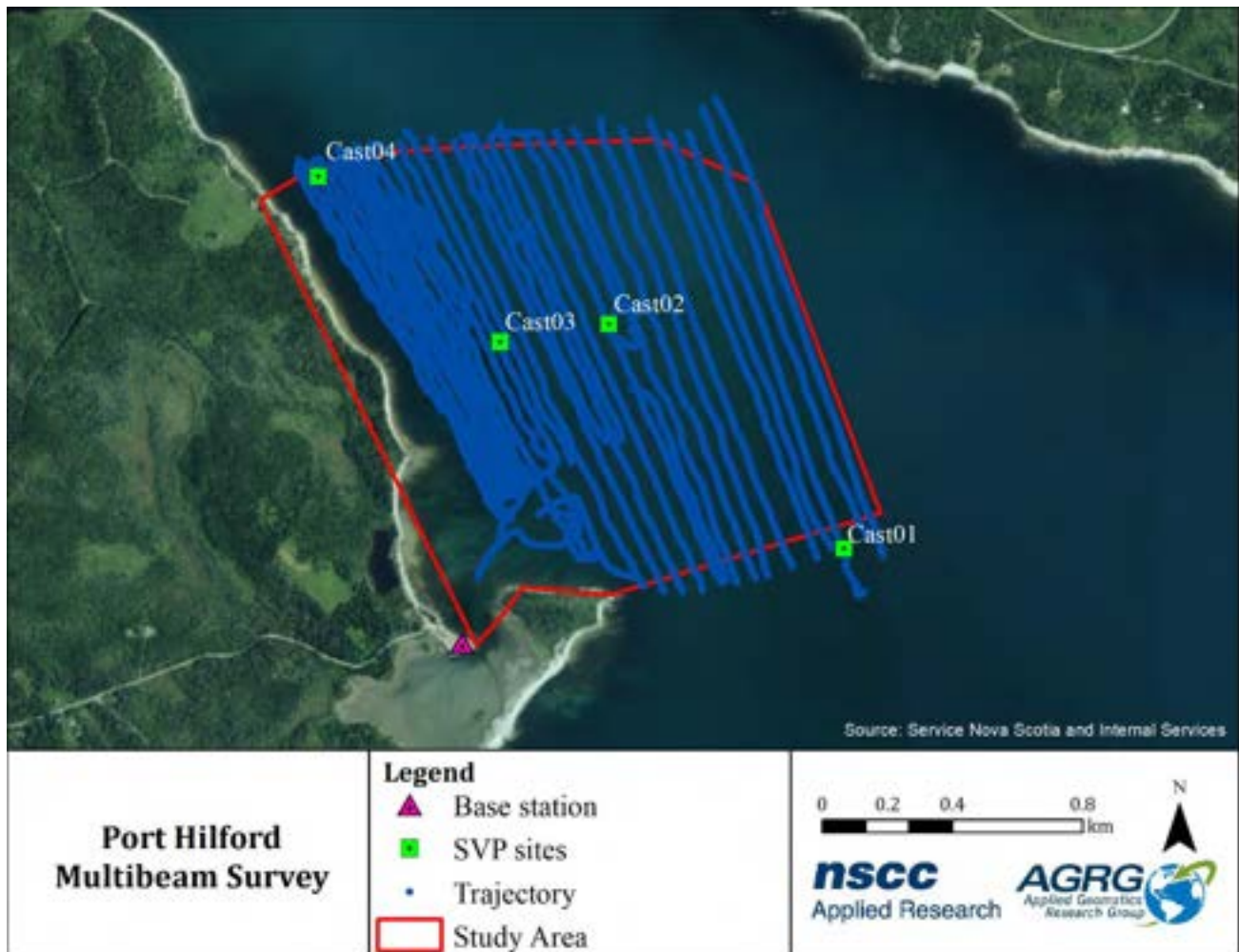
Figure 26 Multibeam survey lines collected on Oct. 22 nd and 23 rd , 2020 along with the Sound Velocity Profile (SVP) drop sites and GPS base station location which was set up on the Barachois wharf.
