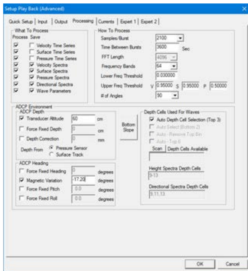
Figure 18 Parameters set up in the processing tab of WavesMon.
