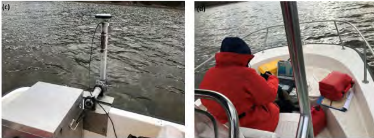
Figure 4.2 a, b Cross sections of the river before and after the Chapel Bridge ( Distance from left bank -downstream) c: GNSS antenna mounted on the pole (port side) above the transducer head d: AGRG researcher collecting echosounder data in Visual habitat software package.
